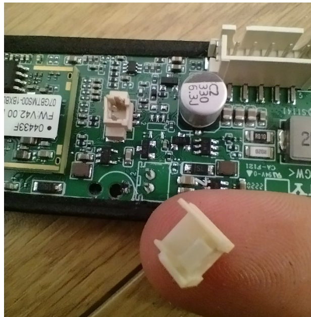
Figure 7, Joseph Shade, Broken SMD mount connector, 2023
